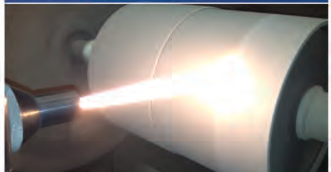
HVOF process deposits WcWoCr coating
