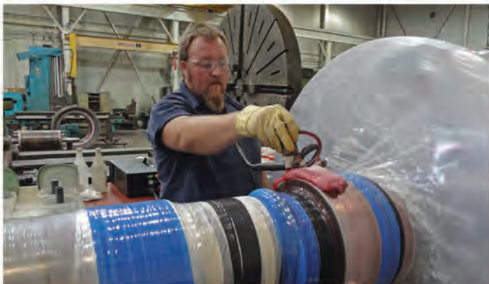
Motor repair with Brush Plating
