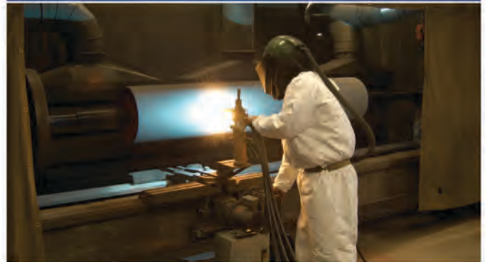
Automated Electric Wire Arc process deposits Wear Coating
